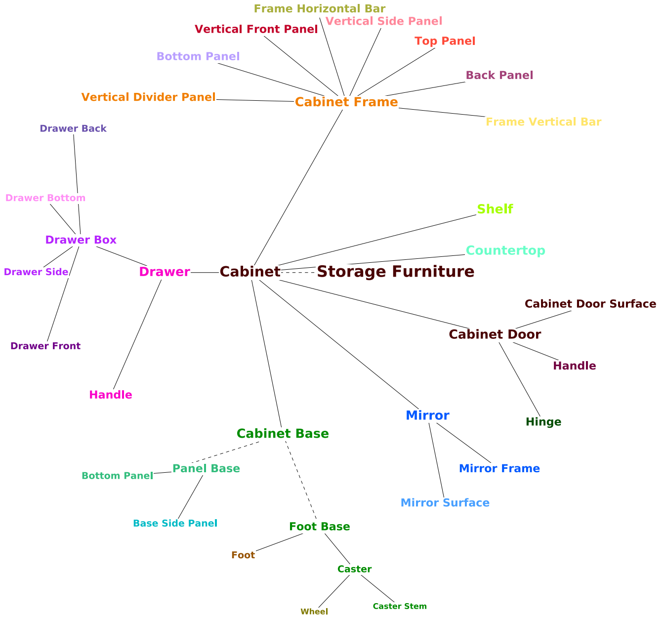
Fig. 5. PartNet semantic hierarchy for storage furnitures. Dash lines show the OR-nodes and solid lines show the AND-node in PartNet. We assign the semantic labels in the figures with the colors that we use for box-shape and point cloud visualization in the main paper.
